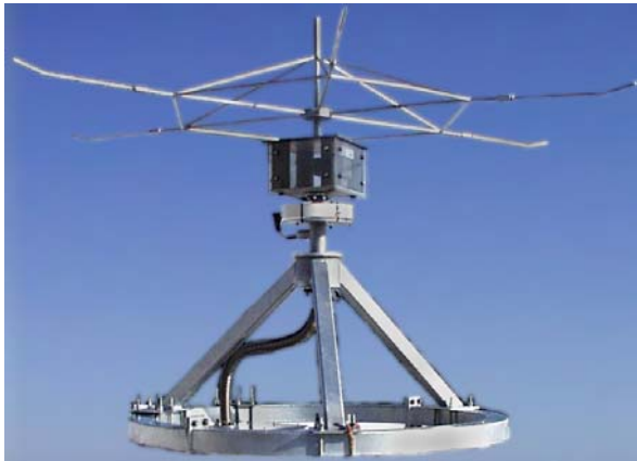
Rogowski Coil installed at the top of tower
