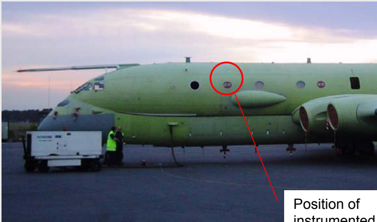
Picture of the window sensor mounted on the window of Nimrod aircraft (photo courtesy BAE Systems)
